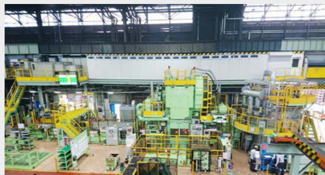
Global standard production line: Integrated line from material heating, to forging, to forging isothermal annealing
