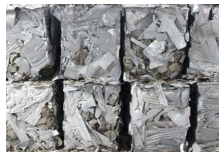
Solid balers Compressed mixture of automotive plant steel scrap (scrap material) and molten solidified material.
