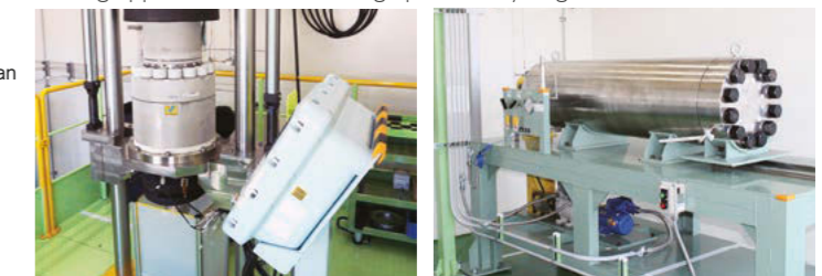
Uniaxial load hydraulic servo apparatus for tensile and fatigue tests (installed 2019)
