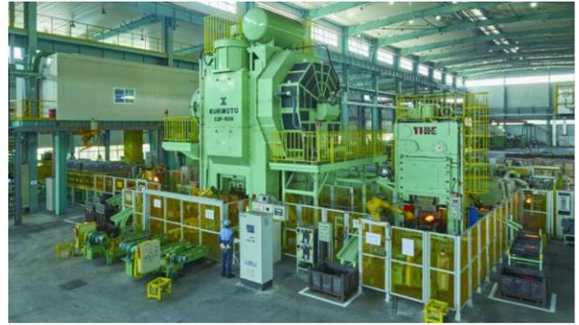
5,000-ton fully automated forging press line
