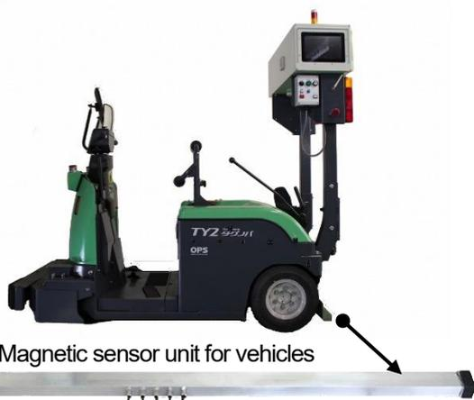
Fig. 2 Magnetic sensor unit for vehicles
