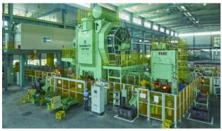
5,000-ton fully automated forging press line
