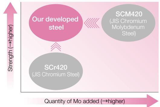
Our newly-developed steel has a strength equal to SCM420 while reducing the quantity of Mo to the level of SCr420.
