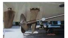
Propeller shaft for ship
