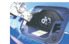
Receptacle on the MIRAI fuel cell vehicle (hydrogen embrittlement resistance)
