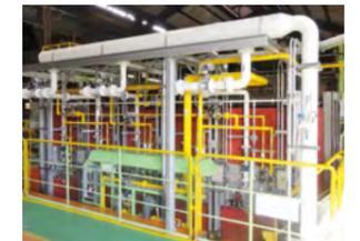
Steel heat treatment furnace with burners installed
