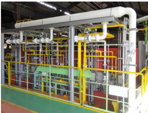
Steel heat-treatment furnace for hydrogen combustion verification trials
